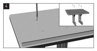
Insert the screws (x4) into the holes on the top plate. Tighten securely.
