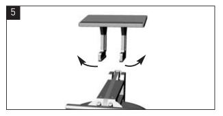
Slightly part the legs of the unit as you place it onto your WaterRower (ensure the ridge on the top plate is on the edge closest to the handle).
