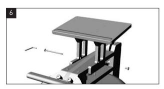
Next, thread the long bolt through the side of the leg. In the hole on the opposite side, insert the nut and tighten securely.
