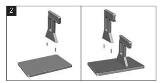
Insert the wooden dowels (x4) into the holes on the top plate. Next, line up the legs with the dowels. Be sure the open 'L'-shaped side corresponds to the ridge on the of the top plate (currently on the underside). See the image of the finished stand to the right for reference. Press the legs onto the dowels until they connect with the top plate.
