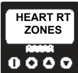
The WaterRower Series III monitor incorporates a heartrate (HR) monitoring facility which requires additional hardware to activate. We highly recommend the use of heartrate monitoring as the most accurate method of monitoring physiological intensity. With the heartrate option fitted, the WaterRower Series III monitor displays heartrate in the stroke rate window 70% of the time.
