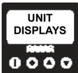
The WaterRower Series III performance monitor allows you to display your workout intensity either as a replicated boat speed in meters per second (m/s), or as Power in watts. It also allows you to monitor average speed or average power of your workout. For many users the units display is not important and for this reason the monitor defaults to the most common unit, m/s.
