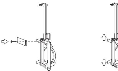
Ensure that the Down Brackets are orientated so the long flat side is on the inside of the rail as shown in the picture below.
