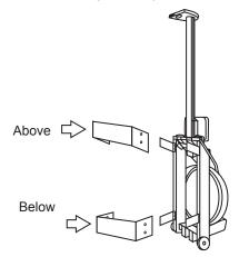
The long, flat part of the Center Bracket should be in a downward position. See pictures below for the correct orientation.
