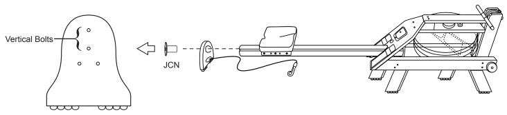
Attach the HiRise Rear Leg to the mono rail, and replace 2 vertical JCNs.
