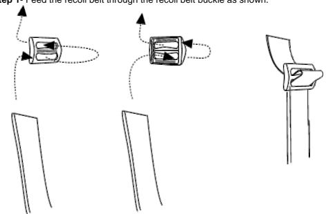
**Step 2-** Feed the loose end of the recoil belt through the d-ring and feed it back on itself through the recoil buckle as shown. Once complete, you may wish to return the loose end of the recoil belt back through the recoil belt buckle for neatness.
